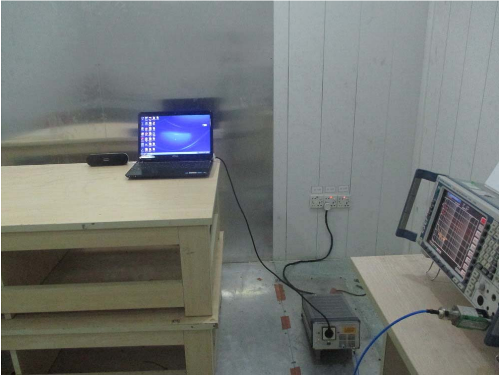
FCC RADIATED EMISSION TEST SETUP
