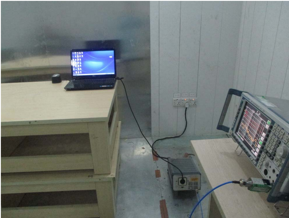
FCC RADIATED EMISSION TEST SETUP
