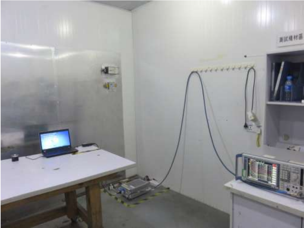
FCC RADIATED EMISSION TEST SETUP
