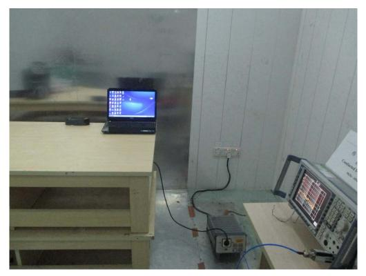
FCC RADIATED EMISSION TEST SETUP
