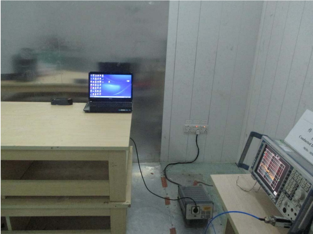
FCC RADIATED EMISSION TEST SETUP
