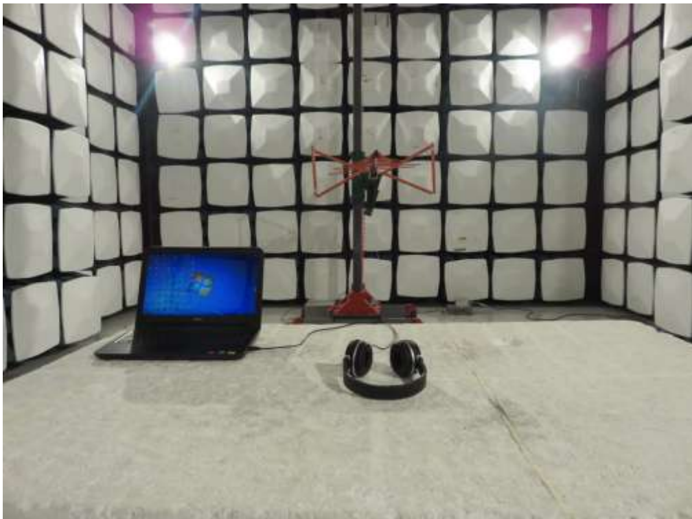
FCC RADIATED EMISSION TEST SETUP
