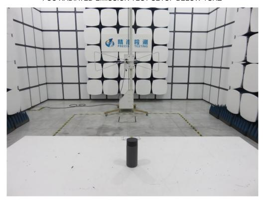
FCC RADIATED EMISSION TEST SETUP ABOVE 1GHZ
