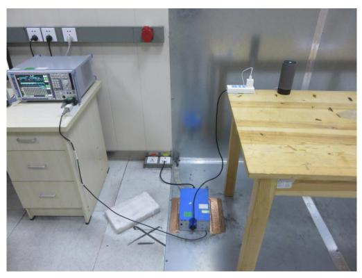
FCC RADIATED EMISSION TEST SETUP BELOW 1GHZ
