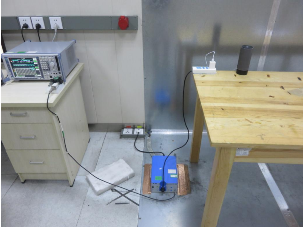
FCC RADIATED EMISSION TEST SETUP BELOW 1GHZ
