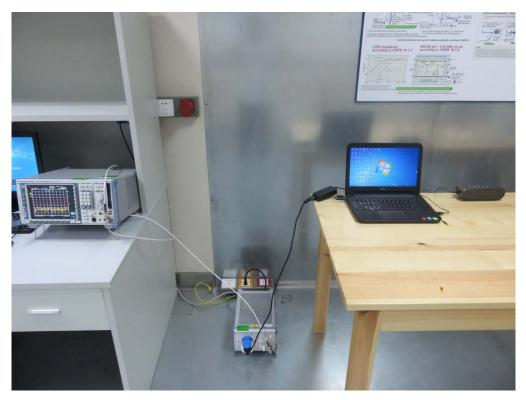
FCC RADIATED EMISSION TEST SETUP
