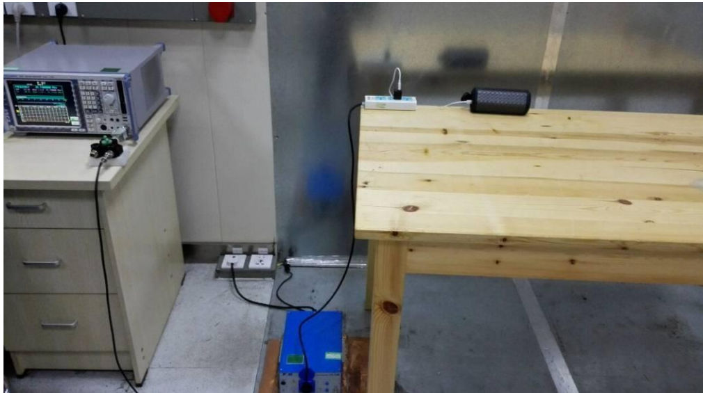
FCC RADIATED EMISSION TEST SETUP
