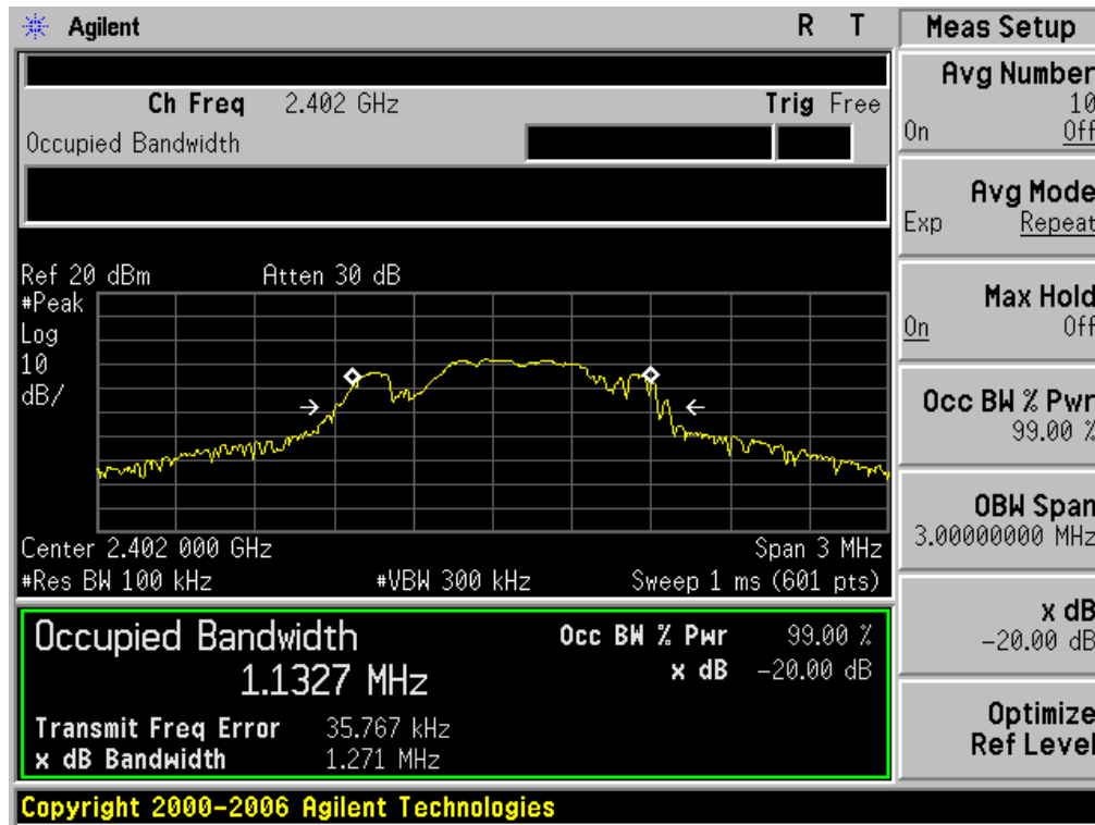
TEST PLOT OF BANDWIDTH FOR LOW CHANNEL
