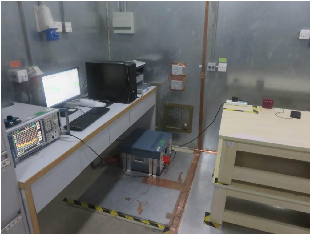
FCC RADIATED EMISSION TEST SETUP
