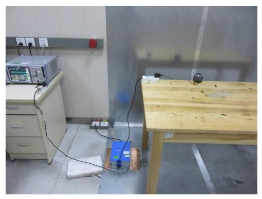
FCC RADIATED EMISSION TEST SETUP
