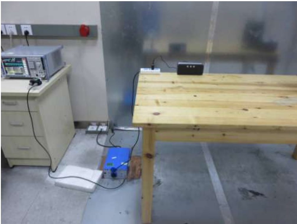
FCC RADIATED EMISSION TEST SETUP
