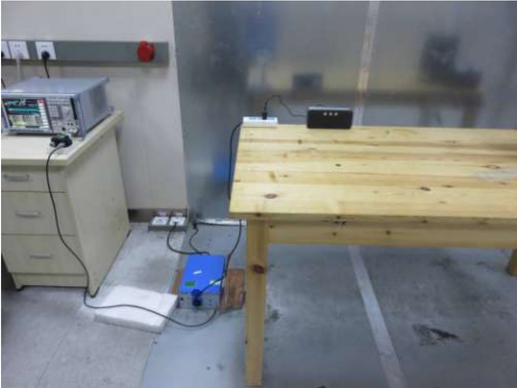
FCC RADIATED EMISSION TEST SETUP
