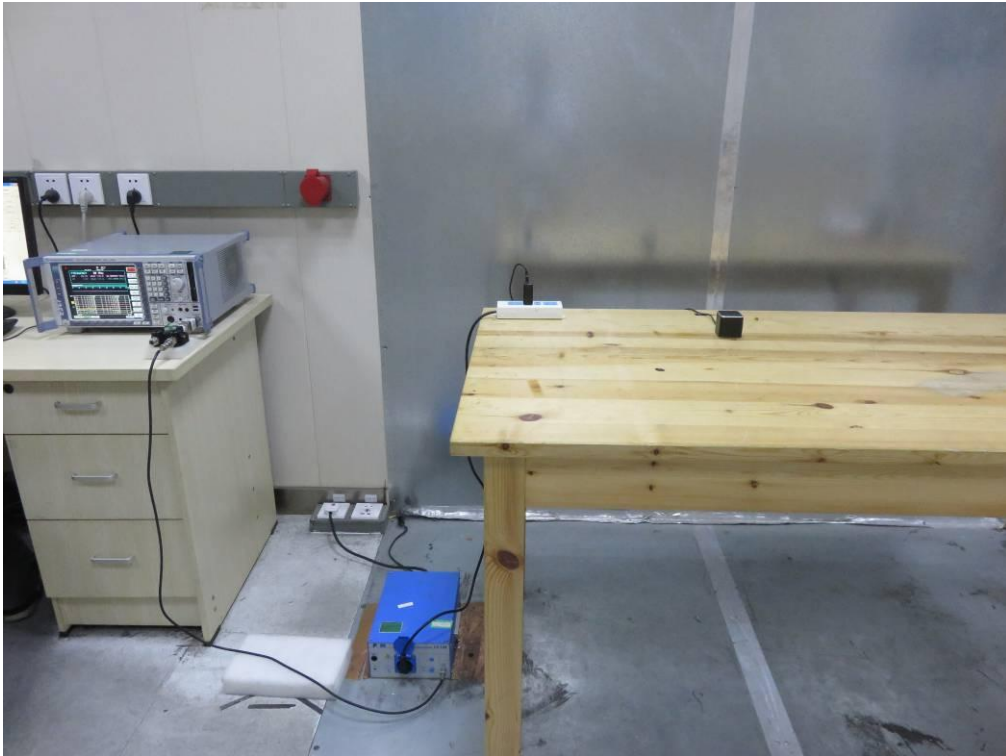
FCC RADIATED EMISSION TEST SETUP
