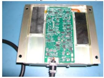
Photo of PV2000 receiver PCA mounted in antenna housing.
