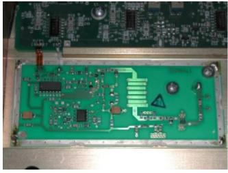
Photo of PV2000 transmitter PCA mounted in antenna housing.
