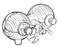
thumbscrew to lock the lamp in place by rotating the screw clockwise. Use caution not to over-tighten the thumbscrew.
