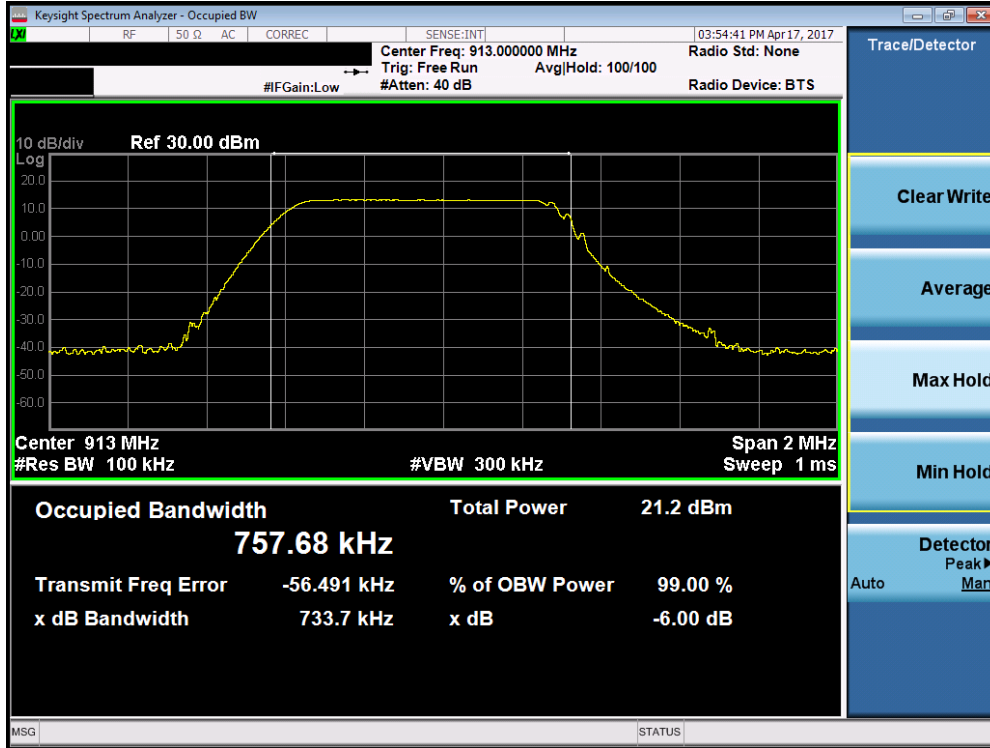
Plot 7-2. 6dB Bandwidth Plot (Mid Channel)
