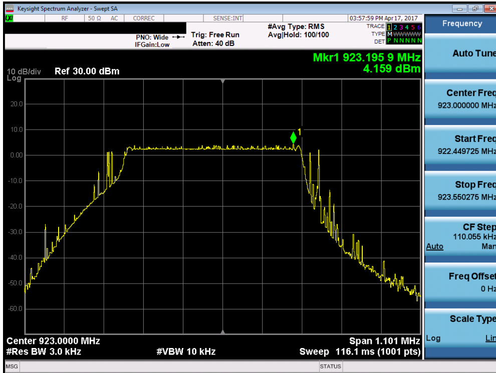
Plot 7-9. Power Spectral Density Plot (High Channel)
