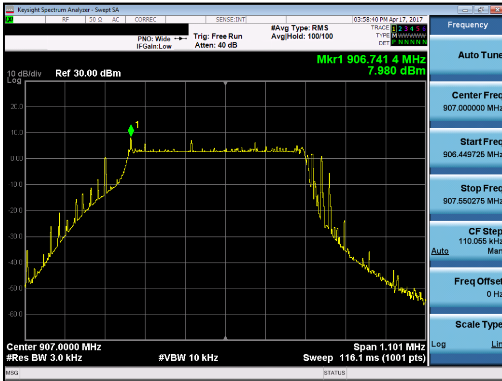
Plot 7-7. Power Spectral Density Plot (Low Channel)
