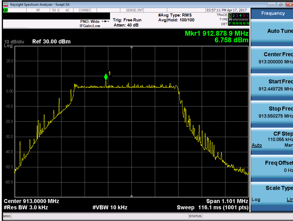
Plot 7-8. Power Spectral Density Plot (Mid Channel)
