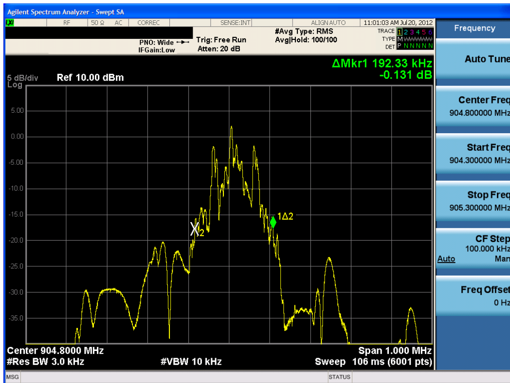
Plot 6-1. 20dB Bandwidth Plot (Low Channel)
