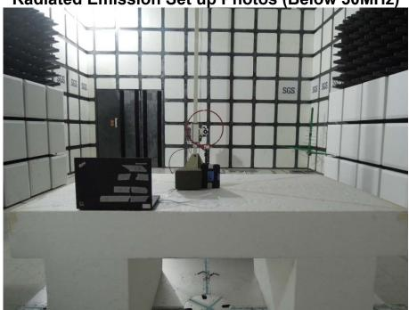
Radiated Emission Set up Photos (Below 1GHz)
