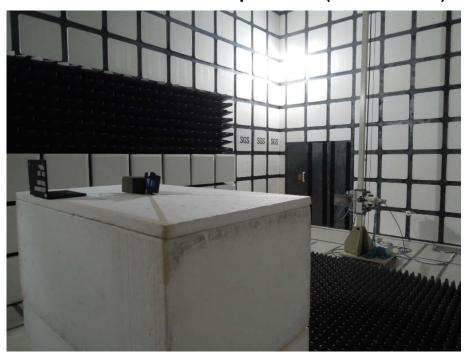
Radiated Emission Set up Photos (Front View)
