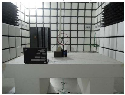
Radiated Emission Set up Photos (Below 1GHz)
