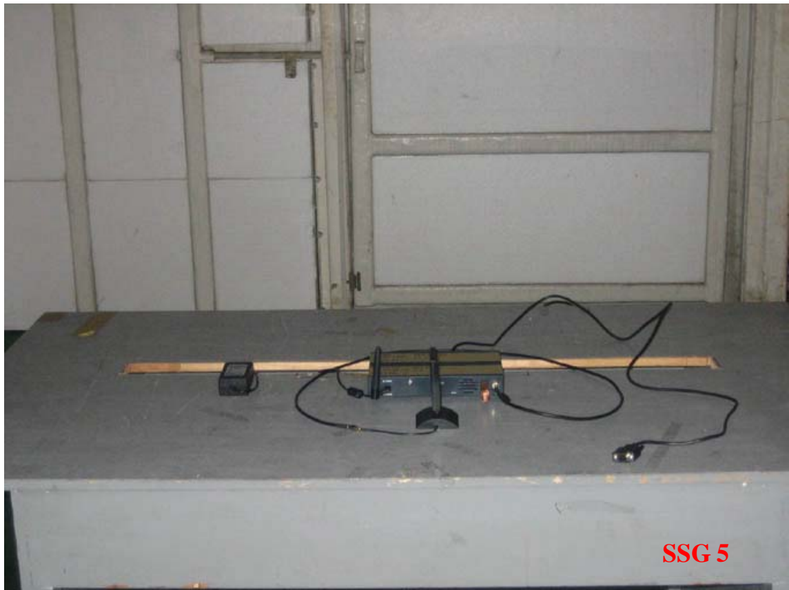
Photo 2: Radiated Emission Test set-up photo
