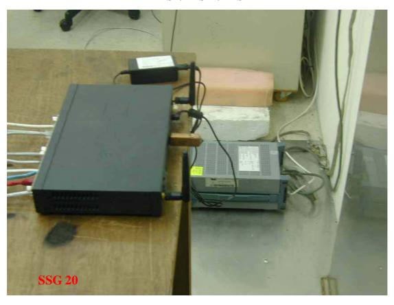
**Photo 3: Conducted Emission Test Set-up photo**
