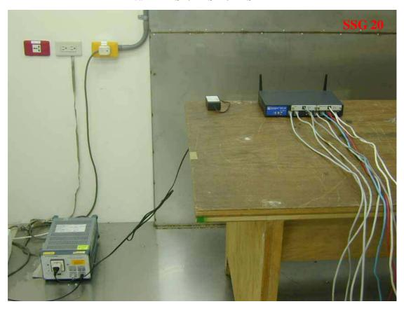
**Photo 4: Conducted Emission Test Set-up photo**
