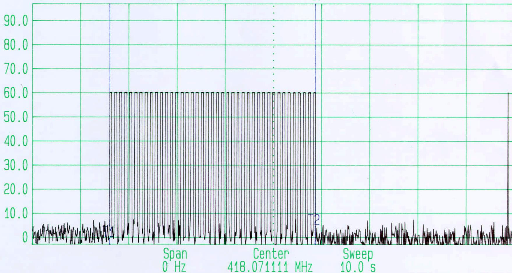
Periodic Timing. Tested By RFI For Crowcon. EUT: Gasman 2. GPH: 40407/02/02/001
