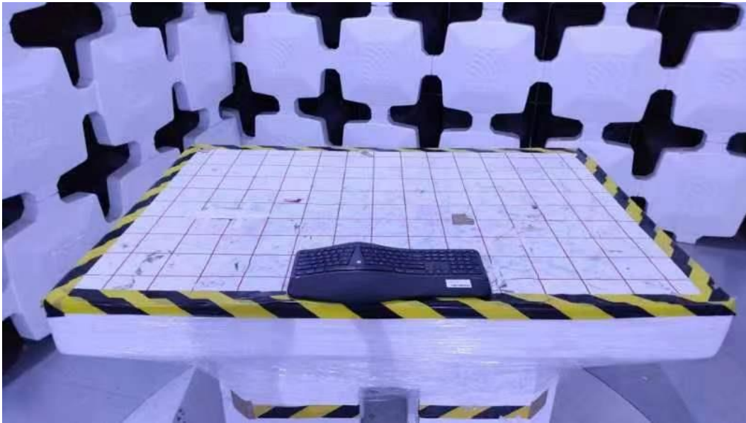
Up to 1GHz The EUT is placed at the center of turntable
