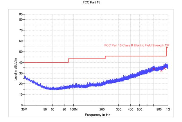
Bandwidth Frequency **QuasiPeak** Meas. **Polarization** Corr. Margin Limit -(MHz) (dBuV/m) Time (kHz) (dB) - QPK QPK (dB) (dBuV/m) (ms) 706.219333 1000.0 120.000 V 33.8 25.4 12.2 46.0 848.971000 32.2 1000.0 120.000 V 25.5 13.8 46.0 916.224333 120.000 V 34.5 1000.0 27.2 11.5 46.0
