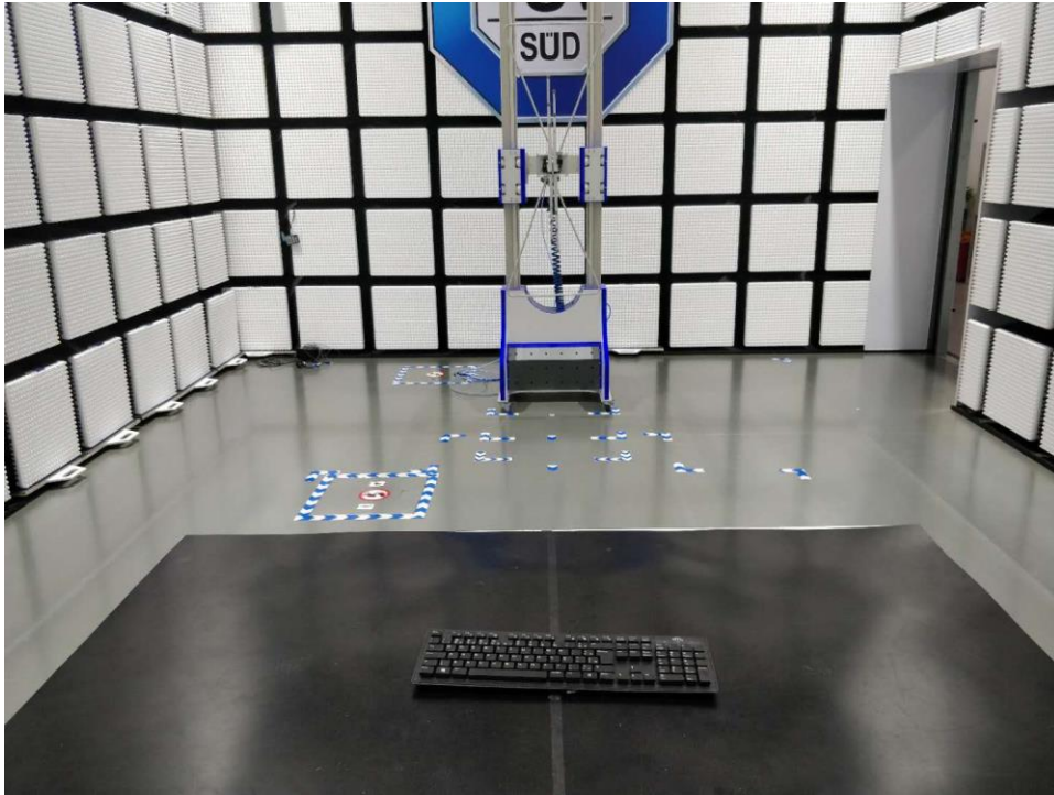
radiated spurious emission 30MHz-1GHz
