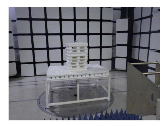
TARGUS SENSOR MODEL: ACS810 BATTERY MODE FCC SUBPART B AND C – RADIATED EMISSIONS – ABOVE 1 GHz
