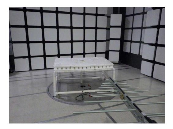
TARGUS SENSOR MODEL: ACS810 BATTERY MODE FCC SUBPART B AND C – RADIATED EMISSIONS – ABOVE 30 MHz
