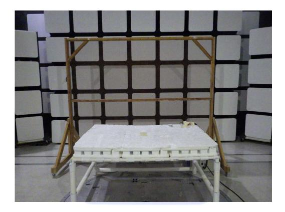
TARGUS SENSOR MODEL: ACS810 AC MODE FCC SUBPART B AND C – CONDUCTED EMISSIONS
