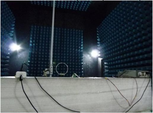
Radiated Emission Set up Photos (Below 1GHz)
