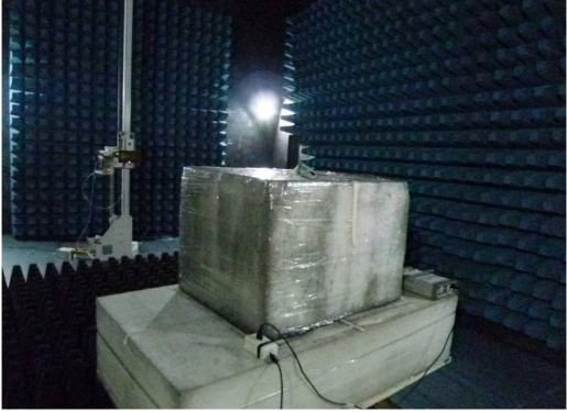
**Radiated Emission Set up Photos (Front View)**
