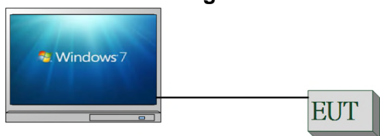
Fig. 2-1 Conducted (Antenna Port) Emission Configuration
