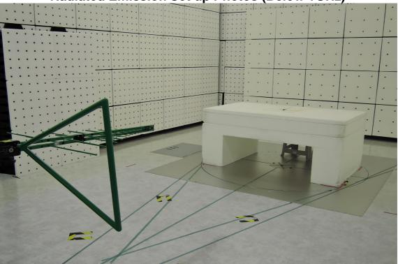
Radiated Emission Set up Photos (Above 1GHz)
