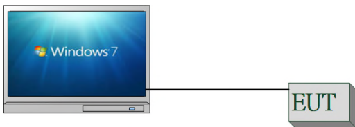
Fig. 2-1 Conducted (Antenna Port) Emission Configuration
