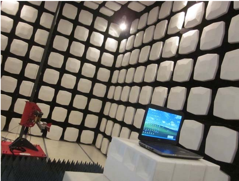
Measurement of Radiated Emission Test Set Up
