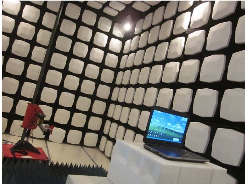
Measurement of Radiated Emission Test Set Up
