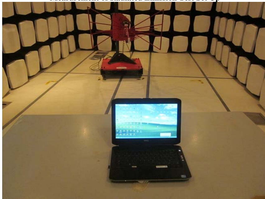
Measurement of Radiated Emission Test Set Up
