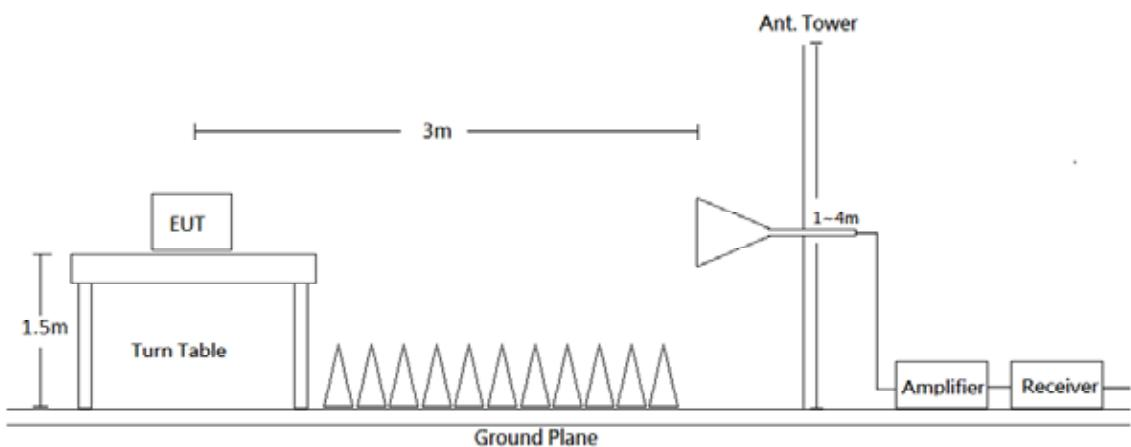
The radiated emission tests were performed in the 3 meters test site, using the setup accordance with the ANSI C63.10-2013. The specification used was the FCC 15.209, and FCC 15.249 limits.
