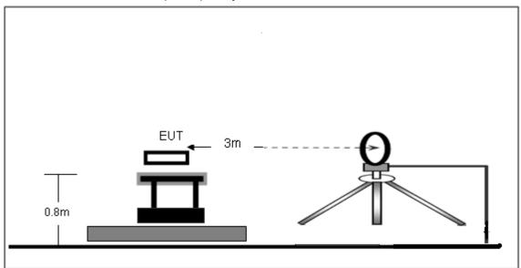
(B) Radiated Emission Test-Up Frequency 30MHz~1GHz
