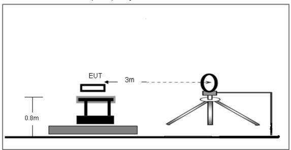
(B) Radiated Emission Test-Up Frequency 30MHz~1GHz
