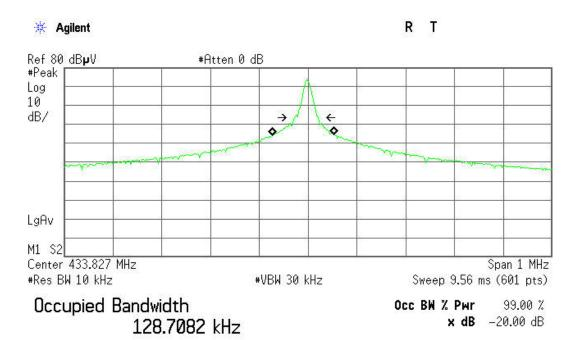
Transmit Freq Error -9.763 kHz x dB Bandwidth 50.396 kHz
