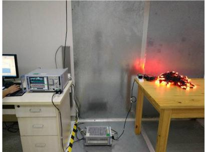
Radiated Spurious Emissions Test Frequency From 30MHz-1000MHz
