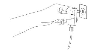
1. Connect the power adapter to the laser light projector. The adapter input voltage is AC120V.
