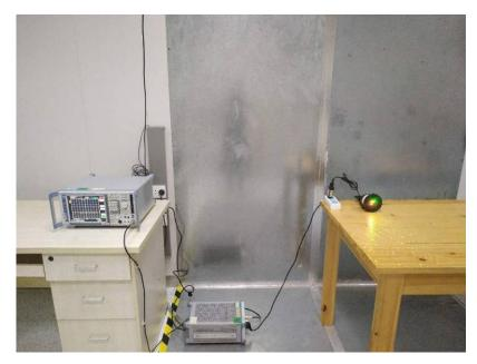
Radiated Spurious Emissions From 30MHz-1000MHz
