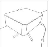
Horizontal orientation: mount the tripod to the bottom of Projector
