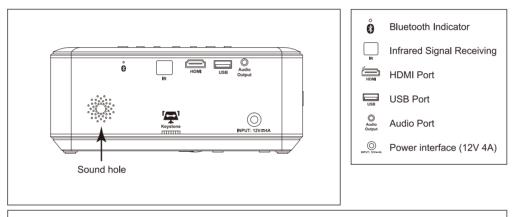
a. Selecting the source by inserting USB, or by connect HDMI cable with your computer or video. b. Connect the speaker through Bluetooth or connect the speaker through the audio cable to output audio.
