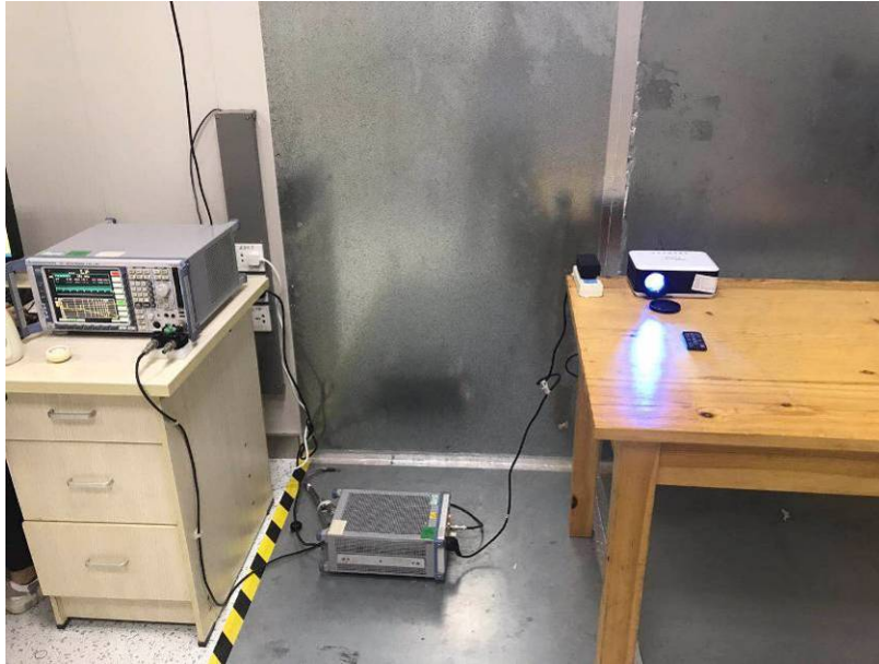
Radiated Spurious Emissions Test Frequency From 30MHz-1000MHz
