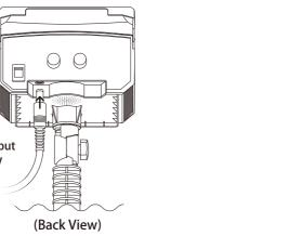
**6** Plug the adapter into an electric socket (AC 120V)
