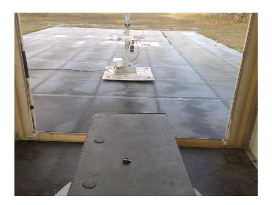
Radiated Emissions Test Configuration 1000-4500MHz
