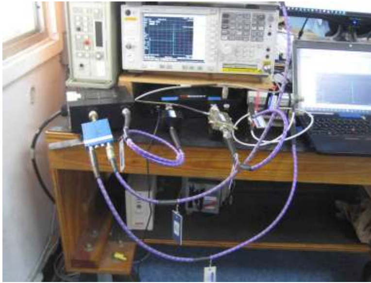
Section 7.11 Oscillation Mitigation (Notch Filter) Test Setup
