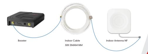
Notes:Plus has built-in antenna so you needn't to install indoor antenna(s),pro is the same situation but if you need more room to be covered ,follow this step(Each HiBoost Plus/Pro series has two additional indoor antennas' port, but it should be noted that if all of them are connected, the built-in antenna will be invalid)
