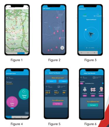
You can also use the "Network Cell Info Lite" to locate the tower and measure the signal strength before & after install.
