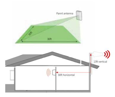
2) After finding the location, hold it there, and watch the gain and power on the App's signal gauge, they shall keep the same or very nearby with the screen shot taken during outdoor antenna install. This is to avoid the loop back between outdoor and indoor antenna(s), please move the indoor antenna till you get unchanged or slightly changed gain and power. This step is quite crucial for the booster's best performance.
