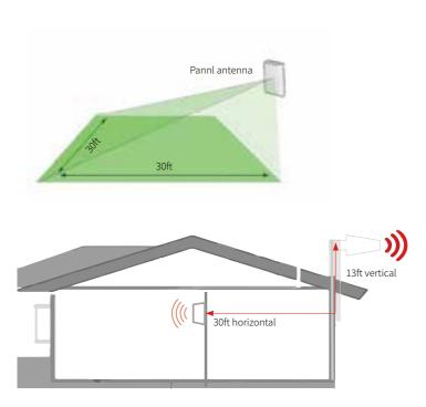
2) After finding the location, hold it there, and ask the other person to compare the gain and power on LCD signal meter, they shall keep the same or very nearby with the photo taken during outdoor antenna install. This is to avoid the loop back between outdoor and indoor antennas, please move the indoor antenna till you get unchanged or slightly changed gain and power. This step is quite crucial for the booster's best performance.
