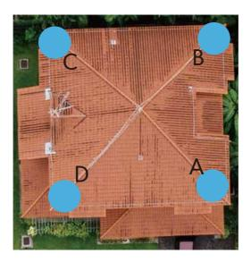
The outdoor antenna needs to maintain a clear line of sight with the cell tower. And it is necessary to avoid the roof or other stuffs from blocking the outdoor antenna.
