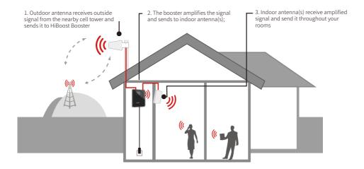
Vice versa,booster(plus)/indoor antenna receices cellphone signal and sends to the booster The booster then amplifies the signal and sends it to outdoor antenna
