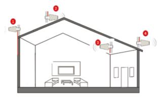
The outdoor antenna needs to maintain a clear line of sight with the cell tower. And it is necessary to avoid the roof or other stuffs from blocking the outdoor antenna.
