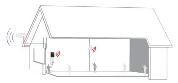
4.2 Connect the indoor antenna with the booster's indoor 1 port by indoor cable, and switch on the booster.
