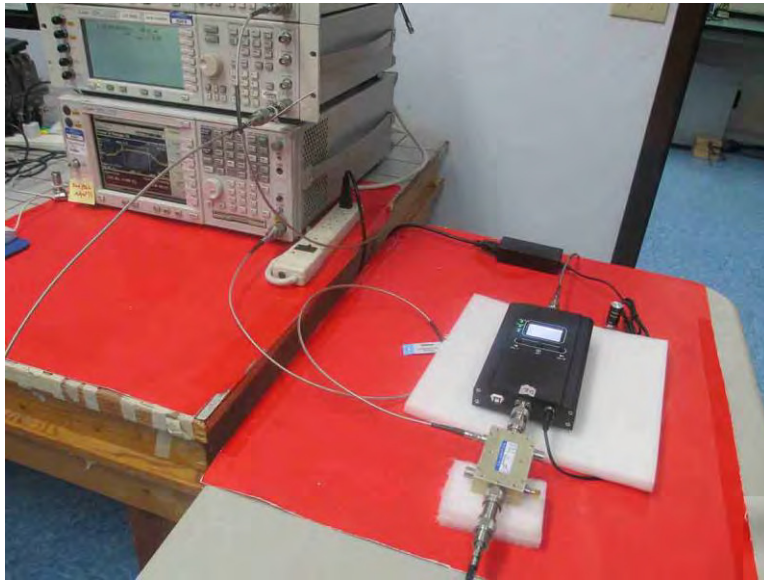
Section 7.9.2 Variable Gain Test Setup
