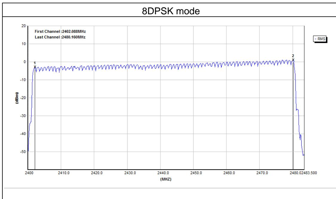
Note: There is a bluetooth device which using FHSS technology, it will be hopping with 79 channel with random sequence. and aslo it could be detect the using channel when the channel was interfered by other devices. the manurfance declare that the bluetooth could use the normal channel was 4,5,6,11,12,16,17,18,36,37,38,39,40,41,42,70,71,72,75,76,77, the device satisfy 15.247 g)& h).
